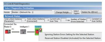
Connect a device station specified as a reserved station to the network.
